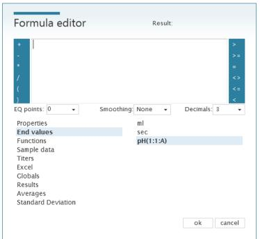
With this function the last measured value is calculated, e.g. a pH value but also a dosed volume using  $\mathbf{ml}$ .
