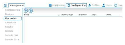
Use  $\oplus$  to add a new electrode. The name is freely assignable (here **Na 61**).
